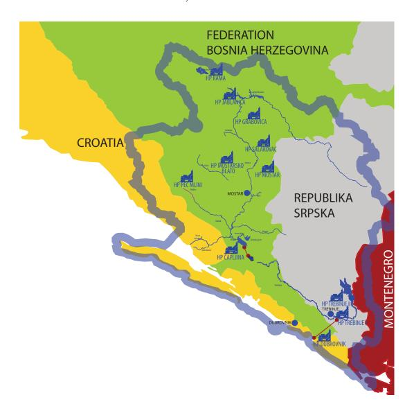
The value of the Trebišnjica hydropower system: Three jurisdictions are operating hydropower facilities in the Trebišnjica basin, sharing about 2.7 billion cubic meters (m3) of water per year and generating more than 2,000 gigawatt hours (GWh) of electricity in 2016. This is about 20 percent of the total electricity supply for Republika Srpska, 9 percent for Federation Bosnia and Herzegovina, and 4.3 percent for Croatia.
